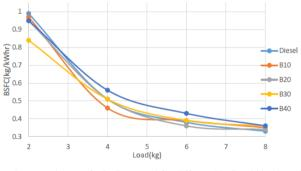
Figure 5: change of BSFC vs Load for different biodiesel blends and diesel
