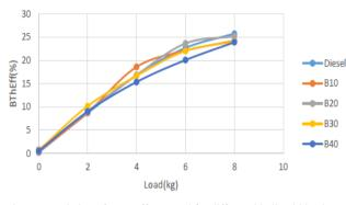
Figure 6: variation of BTH eff. vs Load for different biodiesel blends and diesel
