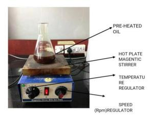
Figure 1: Reactor with magnetic stirrer
