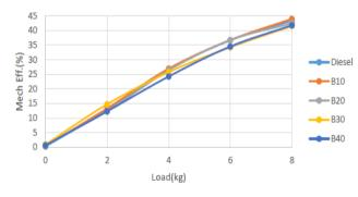
Figure 7: change of Mech Eff. vs Load for different biodiesel blends and diesel
