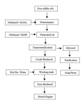
Figure 2: flow chart of two-step transterification process
