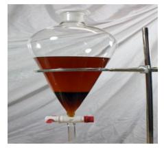
Figure 3: Separating funnel for layer separation
