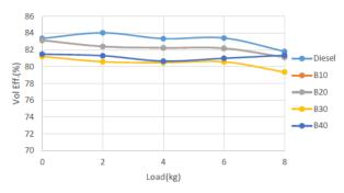
Figure 8: change of Vol Eff. vs Load for different biodiesel blends and diesel
