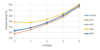
Figure 9: change of Exhaust temperature vs Load for different biodiesel blends and diesel
